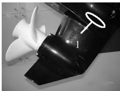
1. Oil level plug screw
