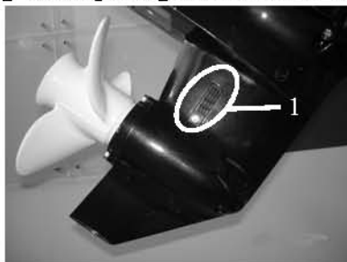
1. Cooling water passage inlet
