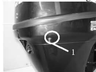
1. Cooling water checking hole
