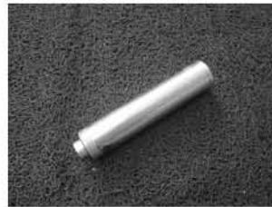
Lower casing cover oil seal installer
