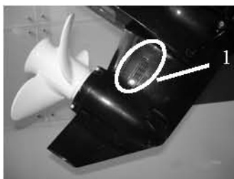
1. Cooling water inlet
