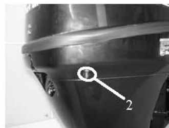
2. Cooling water checking hole
