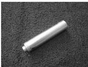
Lower casing cover oil seal installer
