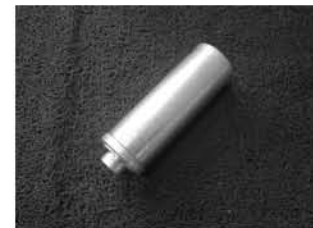
Lower casing cover bearing installer
