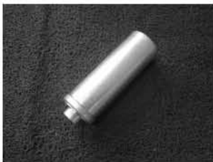
Lower casing cover bearing installer
